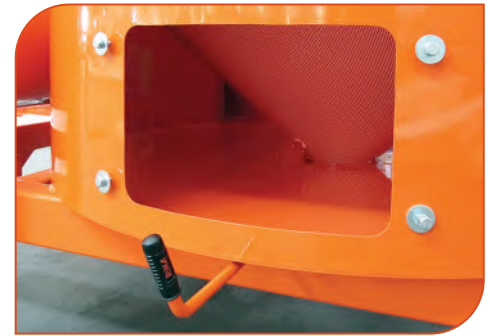
AGD3 can be supplied with different sets of nets for the bottom of silo (2,5 – 4 mm) for drying different kinds of product
